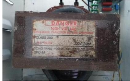
Gambar 20 Microwave Oven Transformer (MOT)
